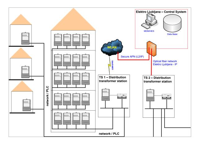
Landis+Gyr measurement data concentrators and industrial & commercial meters with CS / PLC communication interfaces are installed in each of Elektro Ljubljana's transformer stations. The control meters at the transformer station are installed on the secondary side transformer so that the utility can continuously monitor all losses. It can also provide additional quality parameters that give an overview of operations in the utility's entire distribution network.
