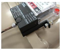
The output device is a magnetically actuated, voltage free reed switch where the electrical instrumentation attached provides the power to detect the opening and closing of the reed switch. The pulse output module is field retro-fittable. The pulse rate output is 1 pulse per 10 litres or 0.01 m3.
