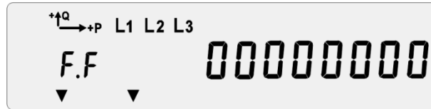
Figure 62 Error message on E650 meters
