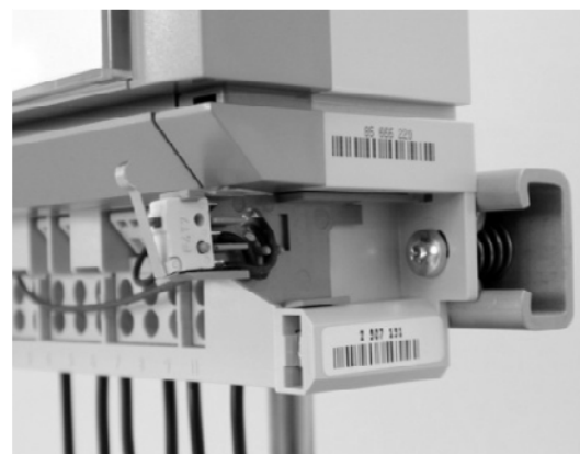
Figure 50 Fixing of cover detection unit to meter
