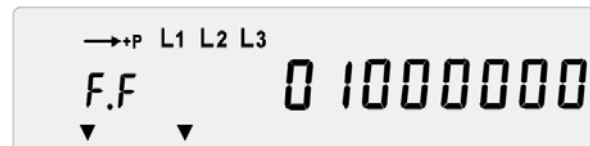
Figure 57 Example of an error message (insufficient battery voltage)
